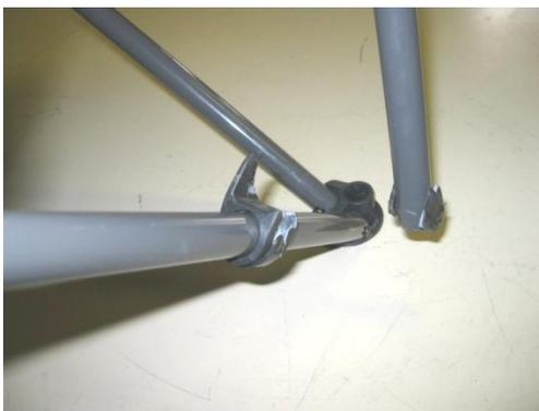
Despite the failures, AFRDI testing staff were surprised at the chair's performance. Tester Guy Manley said: "I really found it hard to imagine that a camping chair could be so strong. OK, it failed in the tests, but this is an accelerated wear testing regime, and the time the chair took to fail represents quite a lot of ordinary use, and by the equivalent of a very heavy man.
