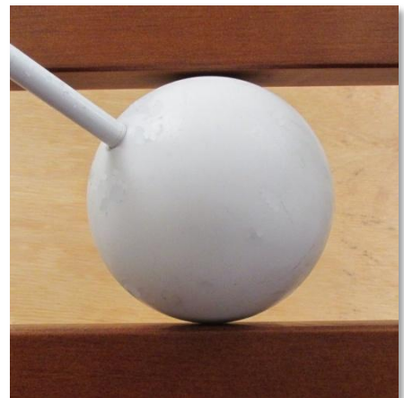
View of a gap failure in a bunk bed side rail.
